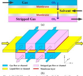
Fig. 1. HASMC configurations (a) Parallel-flow; (b) Cross-flow
