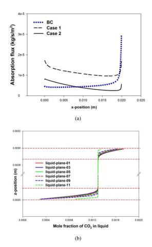
Fig. 2. Parallel-flow HASMC (a) absorption flux; (b) liquid layer concentration profiles (liquid entrance at x=0.02 m and liquidplane-11)
