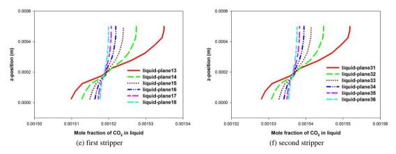
Fig. 3. Cross-flow HASMC mass flux and liquid layer concentration profiles
